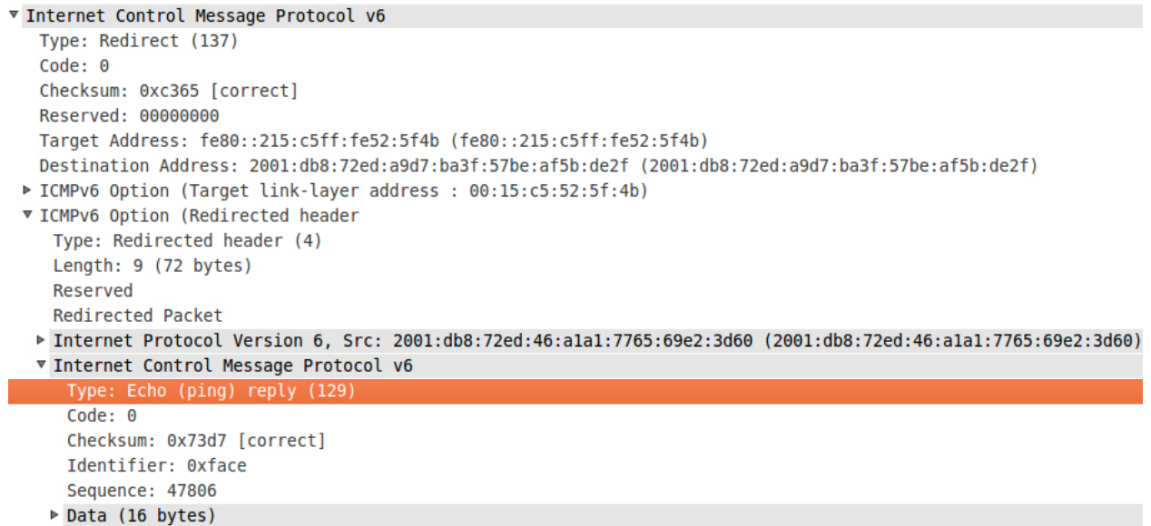
Figure 3.9.: Redirect Spoofing example: the ICMPv6 option “Redirected Header” is filled with the suggested echo-reply from the before spoofed ping-request. (Captured with Wireshark.)
